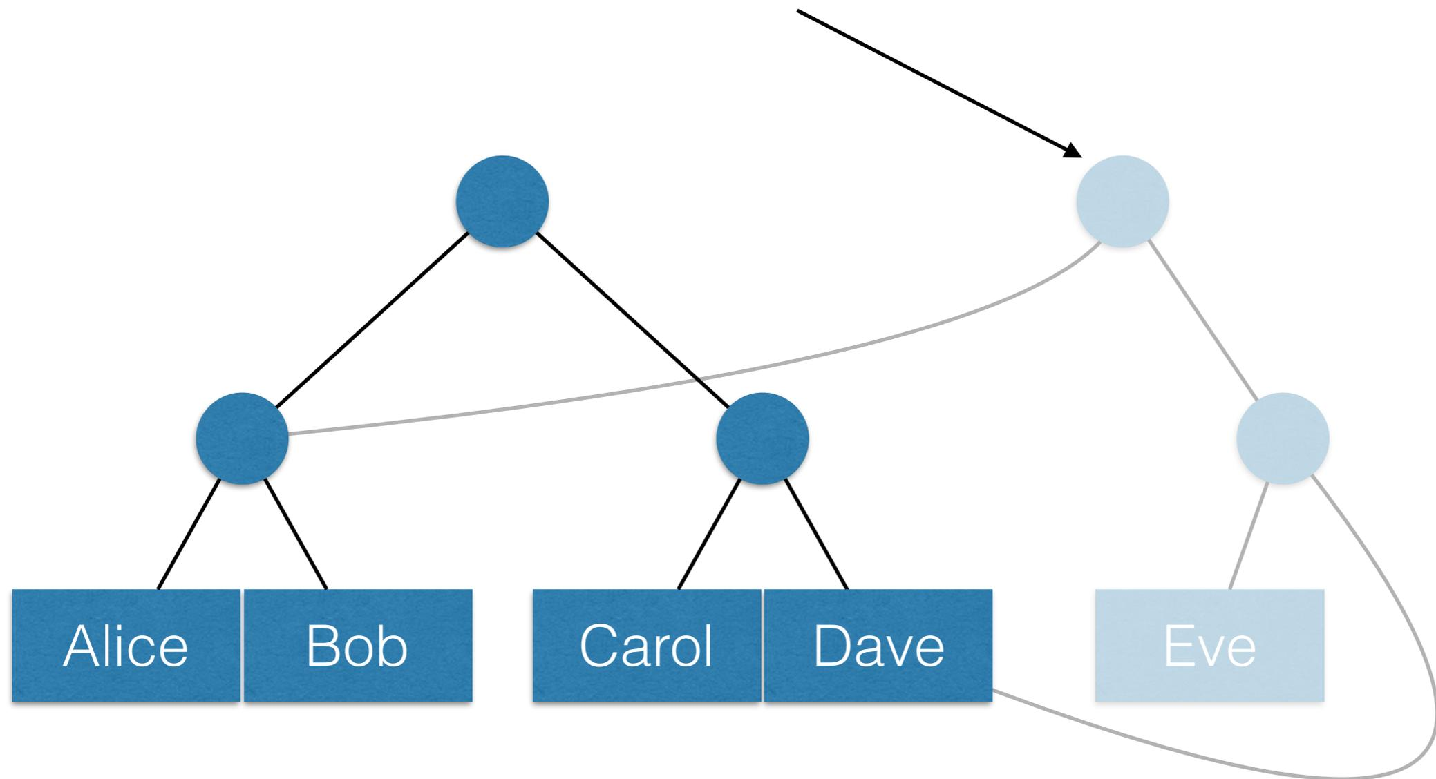
**Data is added, not replaced: No cache coherency problems**
